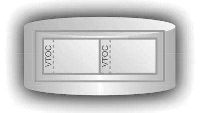
Figure 10-3: A VxVM volume built on subdisks concatenated within the plex and the location of the VTOCs covered by the subdisks (virtual example)
